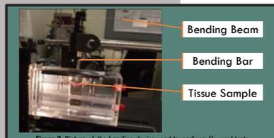
Figure 3: Picture of the bending device used to perform flexural tests.
